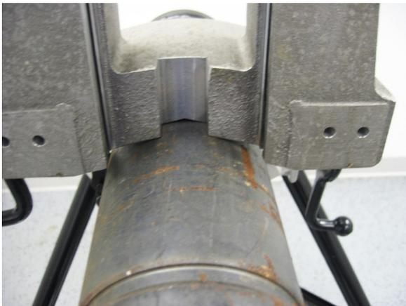
Make sure the machined "V" in the bottom of the frame is centered on the pipe.
