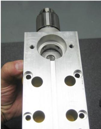
Place lower block on drill with counter-bored hole facing up.
