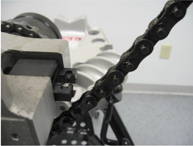
Pull the chain upward and place into the Chain Hook Block #700993. (see below)
