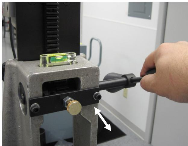
Once the drill has been placed into the frame, hold the feed handle and pull the Retractable Spring Plunger Knob #276899 90 degrees to unlock feed handle before and after drilling.
